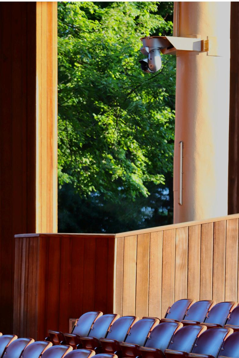
HR140 cameras are mounted on custom designed brackets and attached to the stage walls, and in front of and on the balcony.
